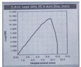
Graph3: 6061-6082 by using circular tip of EN31 tool
