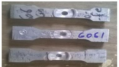
Fig:3 Test samples for Conducting Tensile Strength and Yield Strength
