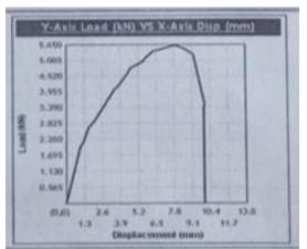
Graph2: 6082-6082 by using circular tip of EN31 tool
